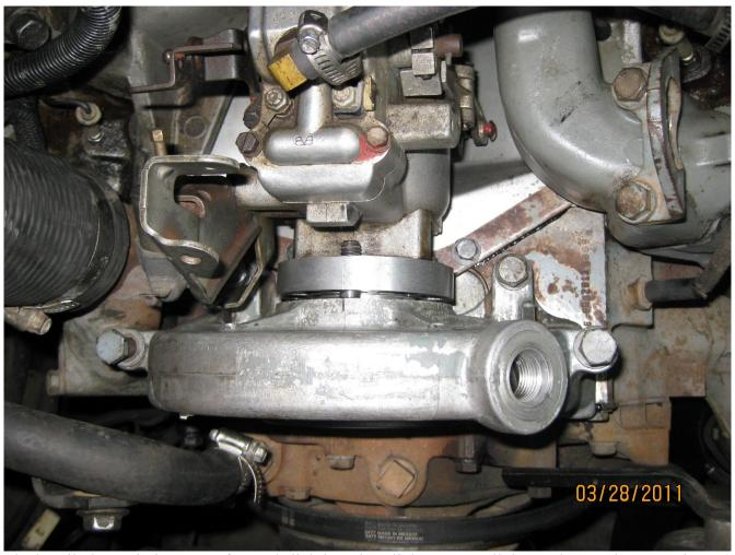
I had to tilt the IP timing cover forward slightly to install the IP. Install the washers and nuts on the IP before fully engaging the IP. Install the IP shaft to timing gear bolts (the 12 point ones). Tighten the timing cover bolts. Now align the timing marks on the IP and timing gear cover.
