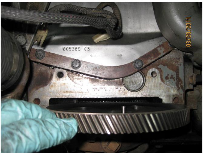
The jiffy marker line should be straight up and down.
