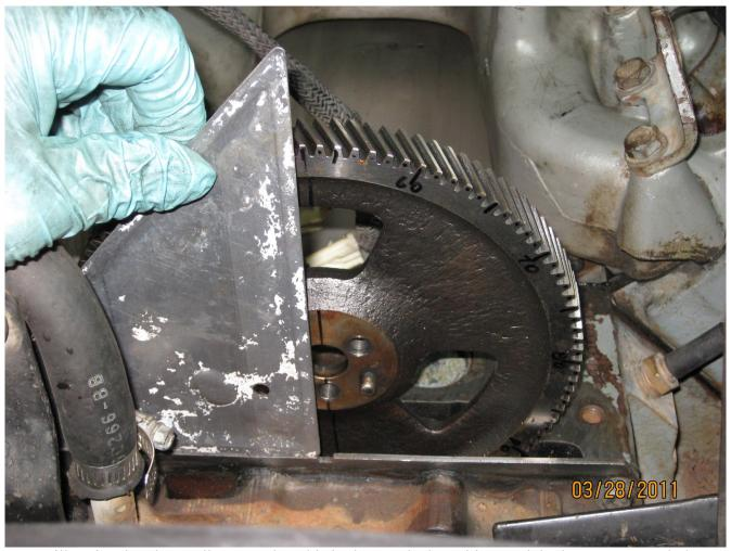
You will notice that the IP alignment dowel is in the 4 o'clock position, and the lower IP pump bolt lines up with the little slot in the timing cover plate.
