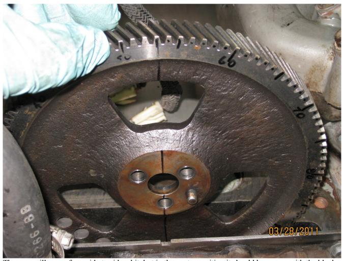
The gear will move from side to side a bit, but in the center position it should be square with the block.
