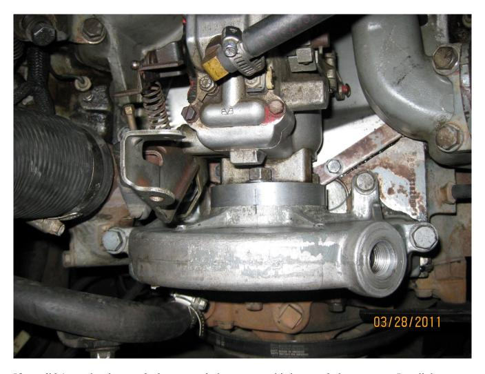
If you didn't previously note the how your timing was set, this is a good place to start. Install the injector lines just snug, remember they will need to be bled. Tighten all the bolts and nuts. Congratulations, you should be able to get the engine started now.
